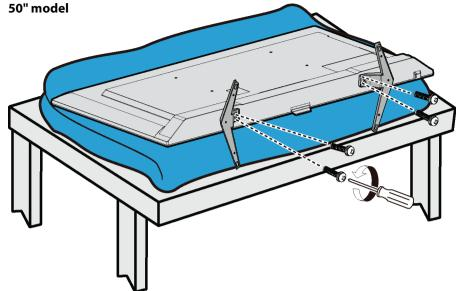
3 Attach the wall-mount bracket to your TV using the mounting holes on the back of your TV. See the instructions that came with the wall-mount bracket for information about how to correctly hang your TV.
