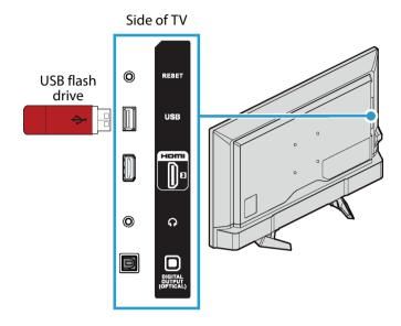
1 Plug a USB flash drive into the **USB** port on the side of your TV.
