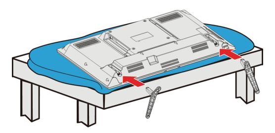
**3** Secure the stands to the TV with the two provided screws.
