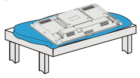
2 Slide the stands into the slots on the back of the TV. Make sure that the long ends of the stands face the front of the TV.
