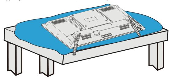
2 If the TV stands are installed, remove the two screws that secure the stands to your TV.
