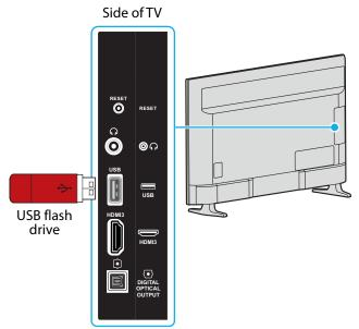
1 Plug a USB flash drive into the **USB** port on the side of your TV.
